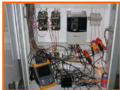
Analyze individual circuits and capture events on equipment or components
